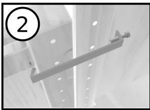
Loosen the fixing screw at the back of the mounting fixture and hook the angled end over the upright.
